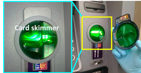
Figure 3: A 3D printed card skimmer acquired during investigation [3].
