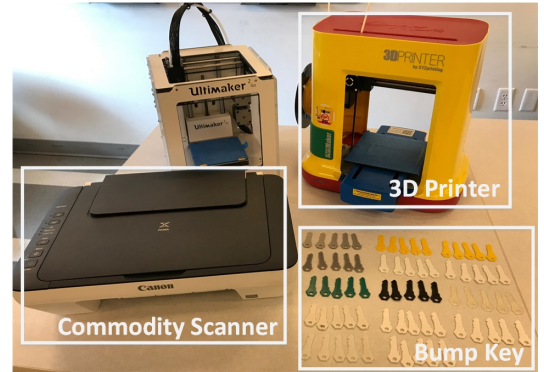
Figure 9: Experimental setup for 3D printer identification where bump keys are fabricated and scanned via a commodity scanner.
