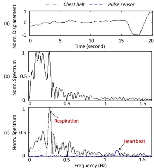
**Figure 9. (a) Twenty seconds time-domain signal under random body motion; (b) Spectrum without random body motion cancellation; (c) Spectrum with the random body motion cancellation, where the blue curve represents the pulse sensor signal and the grey dot dash curve represents the respiration signal.**
