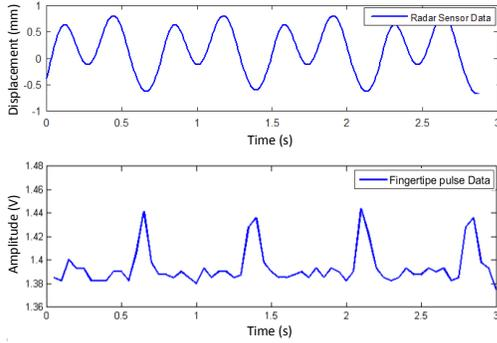
Figure 10. The cardiac motion and the fingertip signal.
