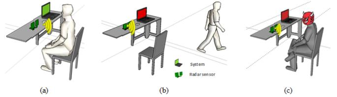
**Figure 7. Continuous authentication scenarios: (a) Authentic user is present, the system remains unlocked. (b) Authentic user leaves, the system locks up. (c) Adversary is present, the system locks up. Green screen means the system is unlocked, red screen means locked.**
