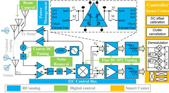
**Figure 3. Doppler radar sensor with adaptive DC tuning and beam control.**
