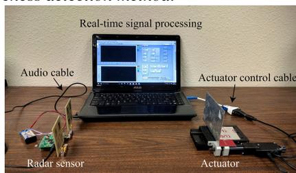
Figure 21. A linear actuator imitates cardiac motion.
