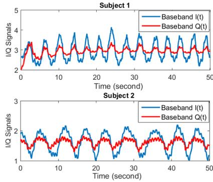
Figure 17. The baseband signals of I/Q from two subjects.
