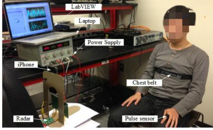
**Figure 8. Experimental setup for cardiac motion sensing.** A subject is sitting one meter away from the radar sensor, and a pulsed sensor was attached to the subject's finger.
